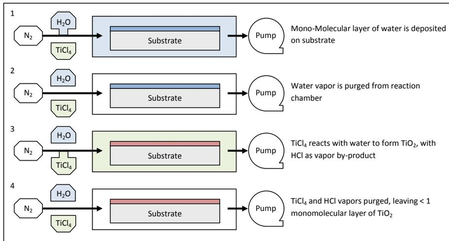
One of these 4-step cycles generates a completed TiO<sub>2</sub> layer which is approximately 0.1 nm thick. For thicker films, the cycle is repeated until the desired total thickness is attained.
